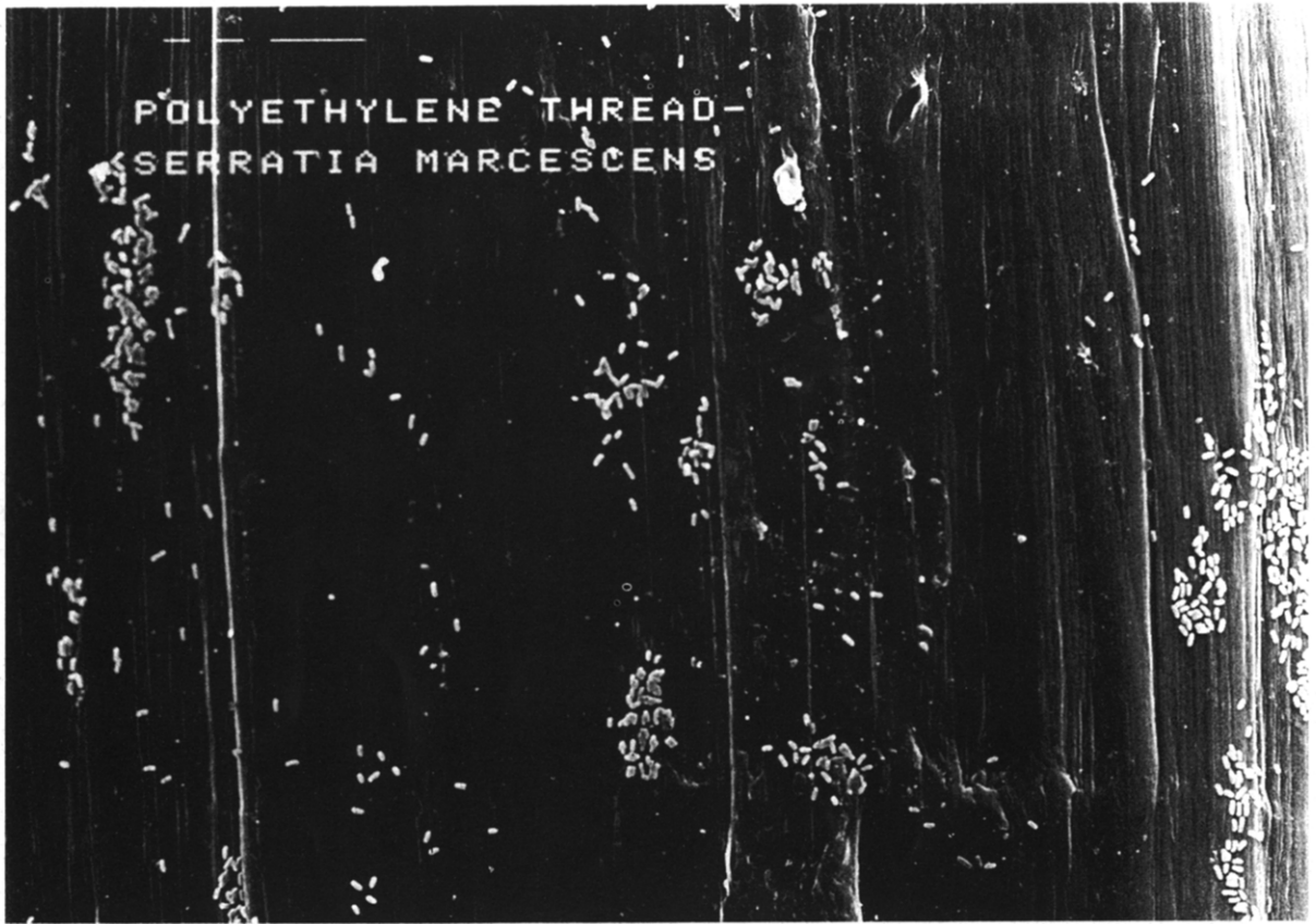
Fig. 5. Se. marcescens adhered to polyethylene thread removed from in vitro model. Section shown is a part of the thread distant from the inoculum reservoir. The cells adhere in discrete clusters.
